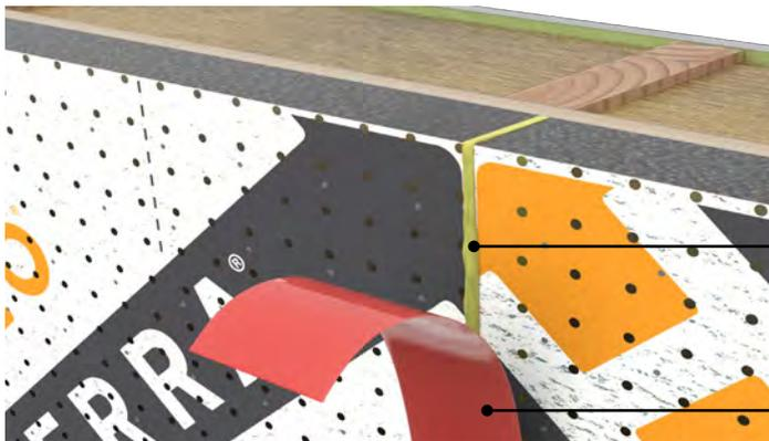
Joints should be tight and snug. Foam fill and tape over joints with gaps 1/16" or larger.
