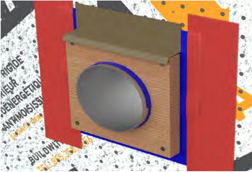
Step 8: Apply sheathing tape to seal edge of membrane and flashing.
