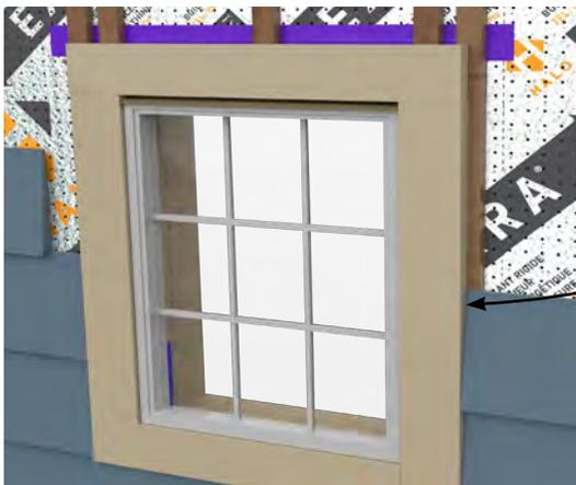
Apply a compatible sealant between cladding and trim boards.
