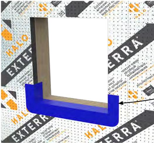
Install a vertical section of the membrane a minimum of 8" up the jamb.
