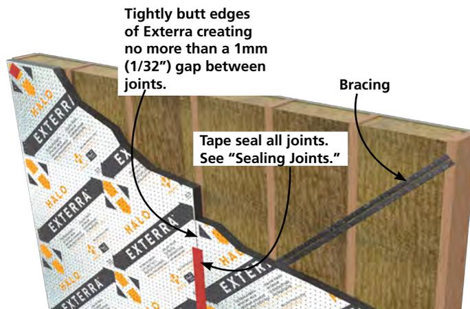
When Exterra is placed over wood sheathing used for corner bracing, furring out the remaining framing members along the wall may be necessary to ensure Exterra sheathing boards are flush with the Exterra sheathing at corners.
