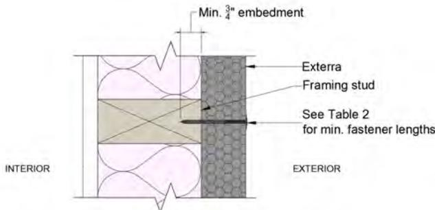
Table 2: Exterra Fastened Direct to Framing Studs
