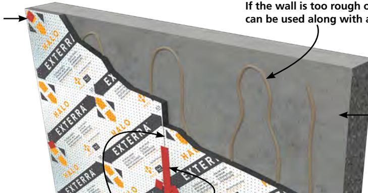
Use weather resistant construction glue compatible with EPS, such as PL 300, to secure Exterra to the wall.
