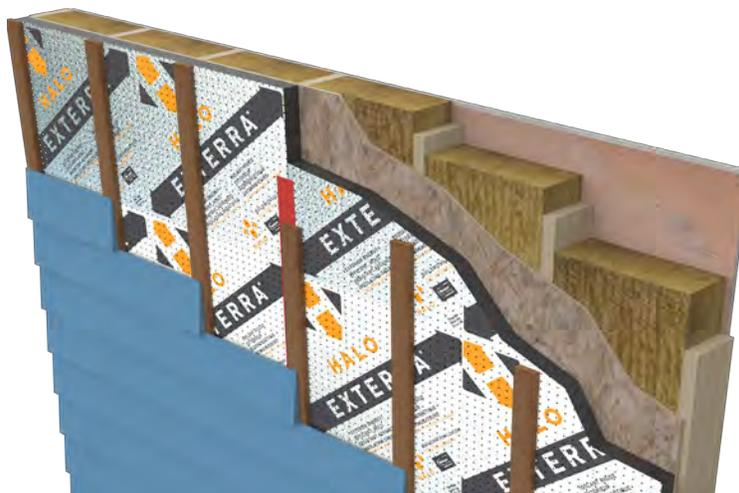
Fasten cladding to the substrate, or if required to the wood furring strips. See Section 8 for fastening information.
