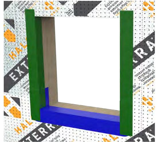
Step 3: Install the flanged window and fasten to the substrate.
