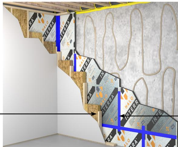
Use construction glue compatible with EPS and concrete, such as PL 300, to secure Interra to the wall. If the walls are too rough or uneven concrete screws with washers can be used along with adhesives to help secure Interra.
