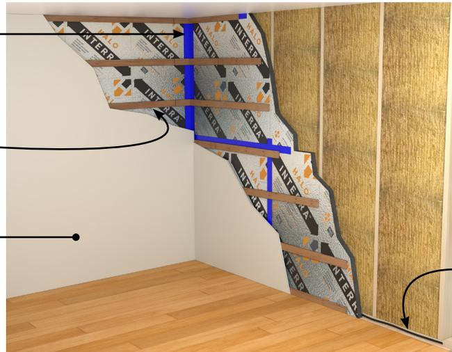
If Interra acts as part of the air barrier system, apply acoustic sealant around the wall perimeter and openings.
