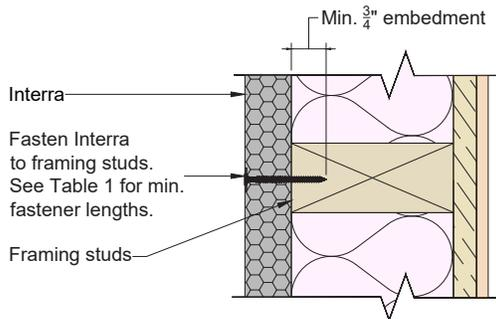
TABLE 1: INTERRA FASTENED TO FRAMING STUDS
