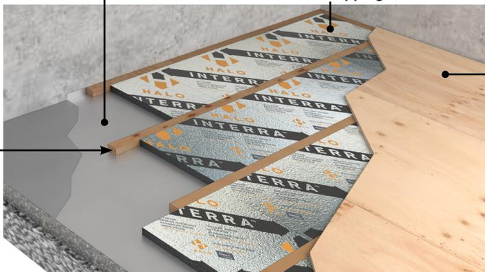
The subfloor is placed over Interra and secured to the wood strapping with adhesive, such as PL 400, and screws spaced at 8" on center. The subfloor should be thick enough to span the wood strappings without significant flexing.
