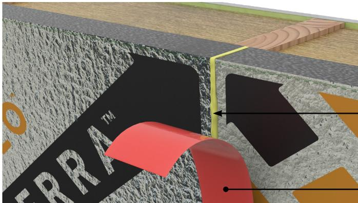
Joints should be tight and snug. Foam fill and vapour barrier sheathing tape over joints with gaps 1/16" or larger.
