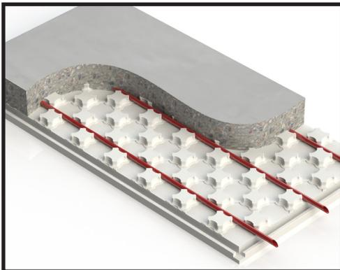
The nodules create a tube channel that accommodates multi-directional placement of 1/2", 5/8", or 3/4" I.D. tubing, with 3" on-center points.
